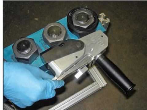
4. Position the insert link on the nut with the reaction foot as close to the contact area as possible.
