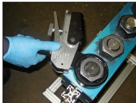
When loose, the wrench can be removed from the nut.
